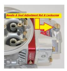
Start the engine and check float level adjustment – The level should be  $\frac{1}{2}$  -  $\frac{3}{4}$  of the way up in the sight window. The level can be adjusted with the nut & lockscrew on top of each bowl.
